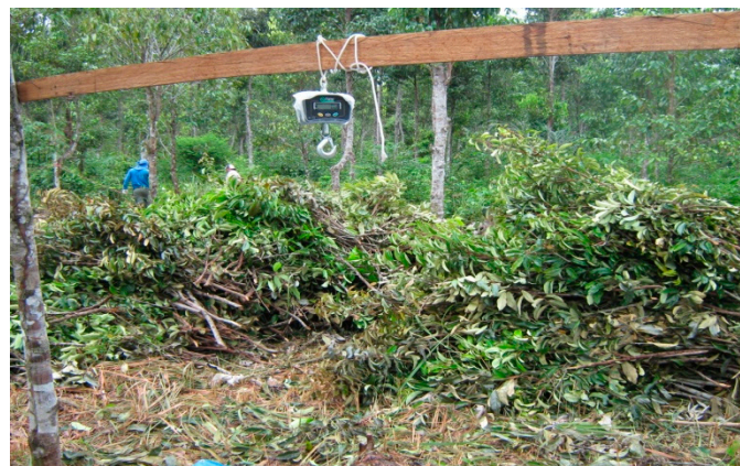
Figure A14. Digital scale for measuring fresh weight of the mass harvested in a rosewood plantation.
