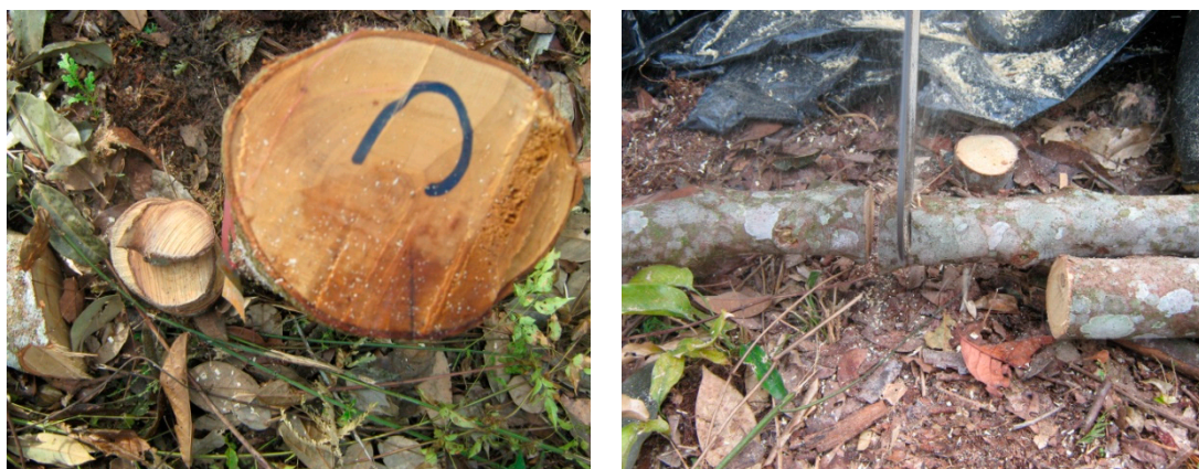
Figure A15. (Left) Collection of wood discs at 0%, 50% and 100% of the height of the stem and (Right) using chainsaws, harvesting sawdust and cutting of the trunk in sections.
